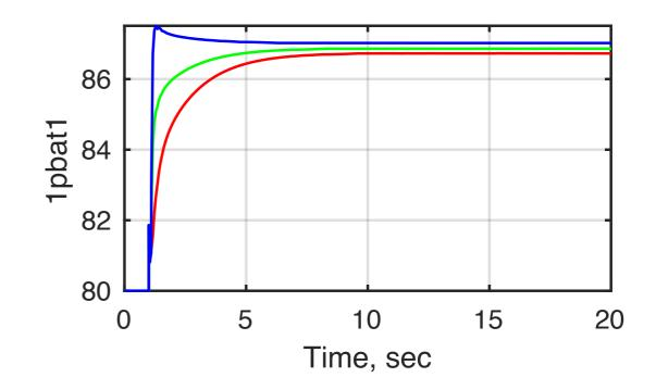
Increase in electronic generation triggered after delay of 100 msec
