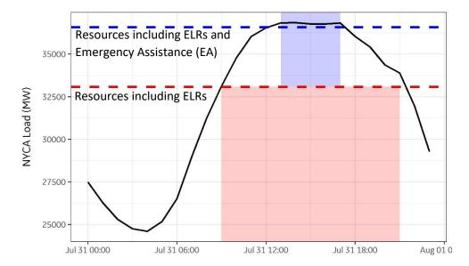
Figure 3. Timing of peak load and EL3/ES dispatch
