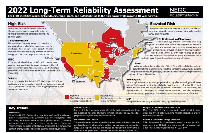
The LTRA highlights five trends: integration of inverter-based resources (IBRs), growth in distributed energy resources (DERs), generation retirements, flat transmission growth and increased demand growth that, without careful planning, could negatively impact the ability of the bulk power system to service the energy needs in North America over the next 10 years.
