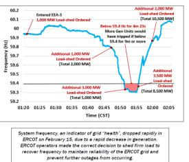
The slide above shows how System frequency, an indicator of grid "health", dropped rapidly in ERCOT on February 15<sup>th</sup>, due to a rapid decrease in generation. ERCOT operators made the correct decision to shed firm load to recover frequency to maintain reliability of the ERCOT grid and prevent further outages from occurring.
