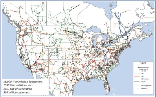
FIGURE 1.3 Diagram of the U.S. high-voltage transmission system. SOURCE: North American Electric Reliability Corporation, 2016, "Critical Infrastructure Protection Committee (CIPC)," presentation March 8–9, https://www.nerc.com/comm/CIPC.
