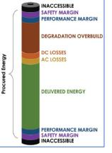
The concept of Degradation Overbuild was of particular interest. Lithium ion BESS have shorter lifetimes than conventional utility generation and transmission and distribution assets. Lifetime expectations often range from 10–20 years (as opposed to 30–50 years for conventional equipment). BESS may experience significant degradation and energy capacity loss over time with usage. Some factors contributing to degradation are:
