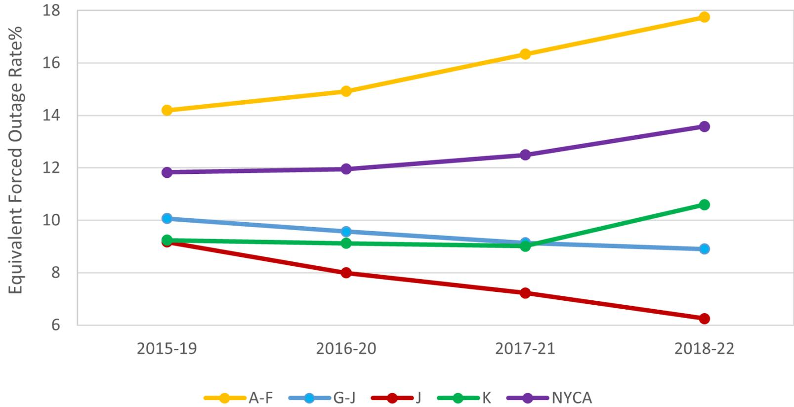
The resources included in the calculation of these values include thermal, large hydro, wind, solar, landfill gas, and run-of-river resources with CRIS.
