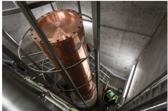
A copper capsule for spent nuclear fuel during a test in the Onkalo spent nuclear fuel repository in Eurajoki, Finland, in 2018
