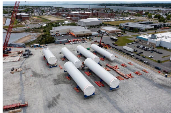
Tower sections for the Vineyard Wind offshore wind farm in New Bedford, Mass
